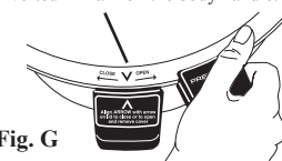
Align the V mark on the cover with the inverted V mark on the body handle.
